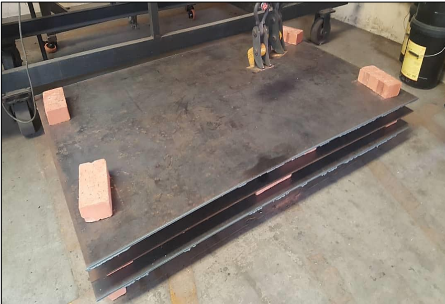
Figure 1: Raw metal plate ASTM A516 Grade 70 carbon steel plate
