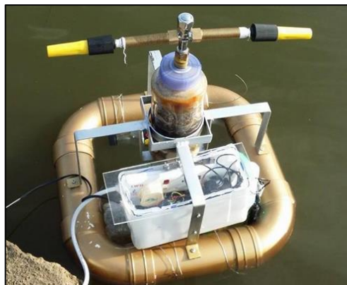
Figure 8: Aerator-IoT device placed on Segment A
