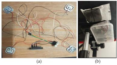
Figure 4: (a) The load cell connection underneath the smart office chair seat and (b) the location of the wiring of the setup
