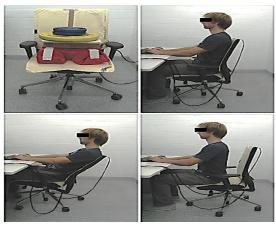
Figure 1: Office chair with the pressure sensor mat on the backrest and the
