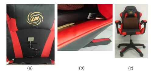
Figure 5: (a) The FSR sensor is attached to the smart office chair and (b) The vibration motor is attached to the smart office chair and (c) The chair ready to be used
