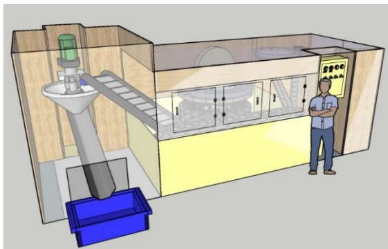
Figure 4: Welding threading machine damper using rockwool
