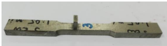
Figure 1: Sub-size dogbone specimen (welded coupon) for tensile test
