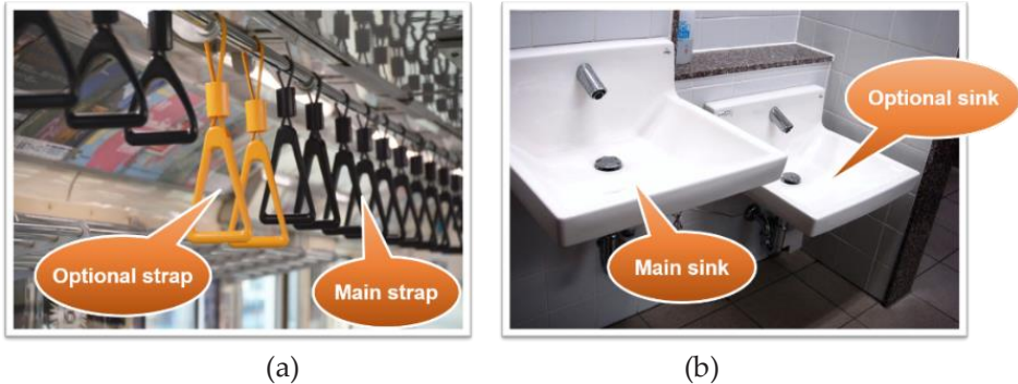
Figure 2: Examples of “low physical effort” products: (a) train straps and (b) restroom hand washing stations
