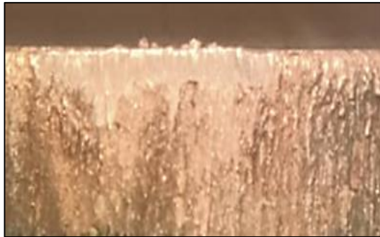
Figure 13: Wear started to develop at the middle of flank area at 363 seconds machining time for 22MnB5 Boron steel cutting tool
