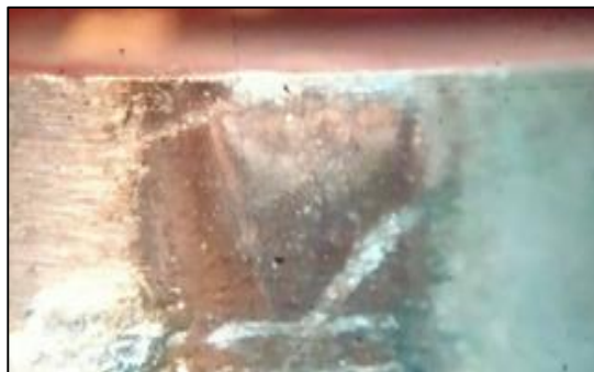
Figure 10: Formation of flank wear at 65 seconds for HSS cutting tool
