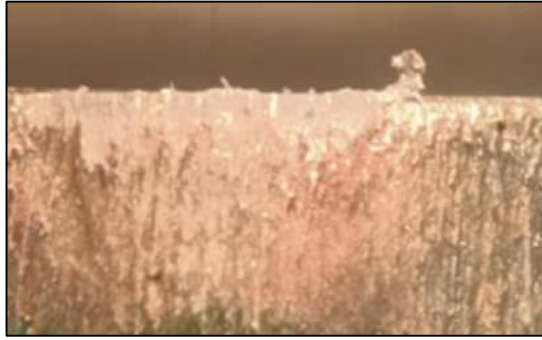
Figure 14: The tribolayer appeared firmly attached to the edge of the cutting tool for 22MnB5 Boron steel cutting tool
