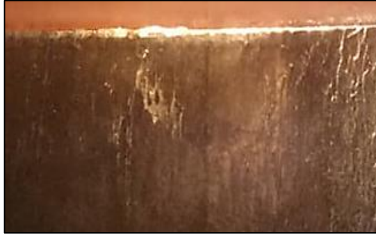
Figure 12: Minor formation of notch and flank wear at 40 seconds machining time for 22MnB5 Boron steel cutting tool
