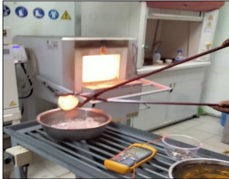
Figure 3: 22MnB5 boron steel sample undergo a rapid water soak for the quenching process
