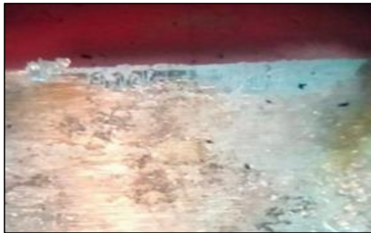
Figure 12: Flank wear increase with small BUE appears for HSS cutting tool
