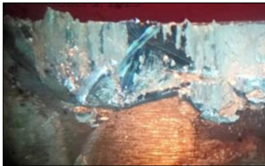
Figure 17: A distinct molten aluminum layer was observed on the wear area at 595 seconds machining, with solidified aluminum visibly adhering to the surface.
