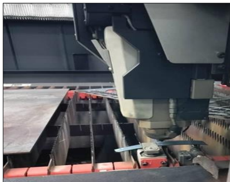
Figure 1: The procedure of cutting a 22MnB5 boron steel sample by a laser cutting machine
