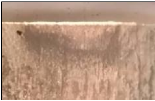
Figure 7: Minor formation of flank wear at 69 seconds for 22MnB5 Boron steel cutting tool
