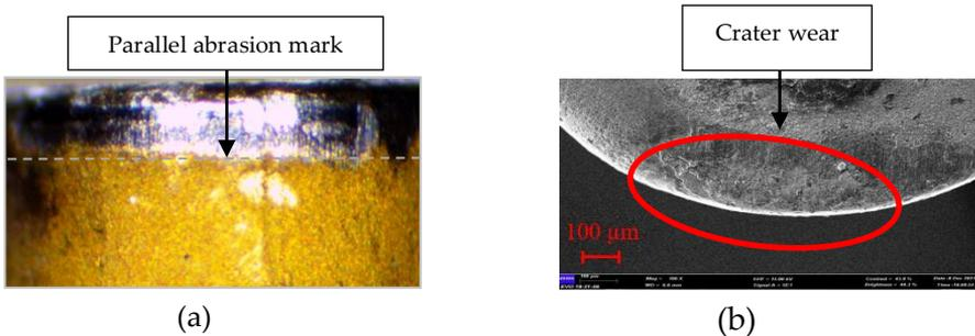
Figure 5: Wear mechanism of (a) front view and (b) top view at 100 m/min Vc and 0.10 mm/rev Fr
