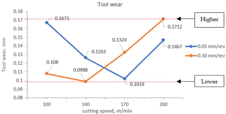
Figure 3: Cutting speed vs. flank wear
