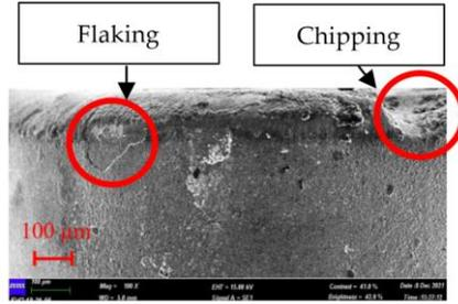
Figure 7: Wear mechanism when a machine at 200 m/min  $V_c$  and 0.10 mm/rev  $F_r$
