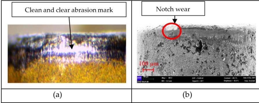
Figure 4: Wear mechanism when a machine at 100 m/min Vc and 0.05 mm/rev Fr with (a) and (b)
