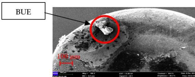
Figure 8: BUE formation on the top view of the cutting tool at the same  $V_c$  and  $F_r$
