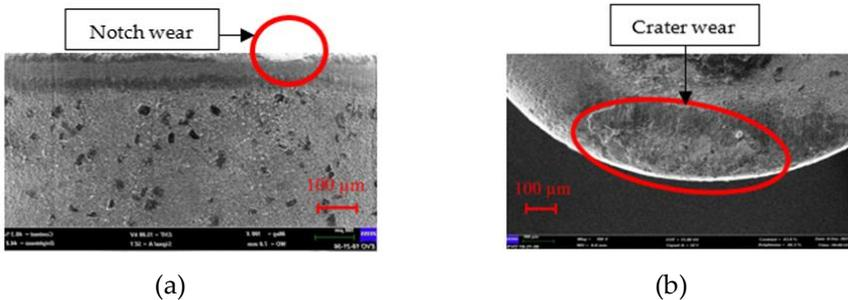
Figure 6: Wear mechanism of (a) front view and (b) top view at 200 m/min  $V_c$  and 0.05 mm/rev  $F_r$
