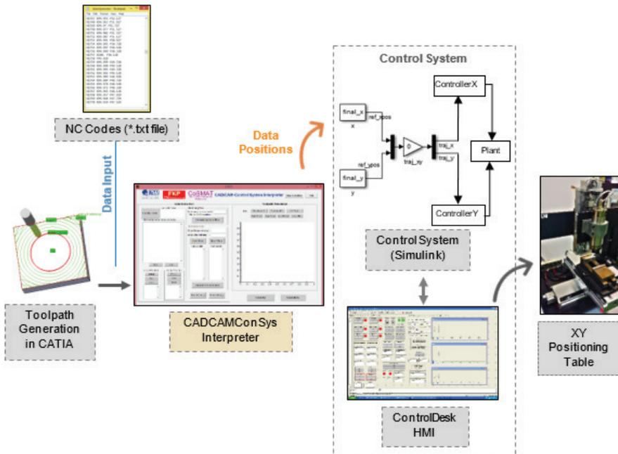
Figure 4: Implementation of CAD/CAM-MATLAB/Simulink interpreter with a milling machine positioning table.
