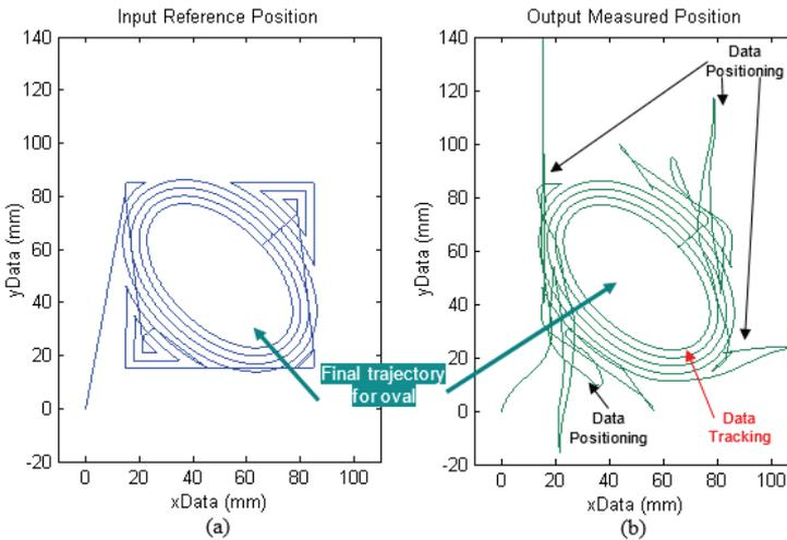
Figure 7: (a) reference tracking and (b) measured tracking data for oval shape contour
