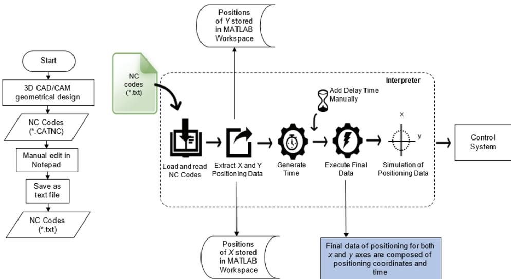
Figure 1: Architecture design of the interpreter
