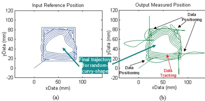
Figure 8: (a) reference tracking and (b) measured tracking data for random-curve-shape contour
