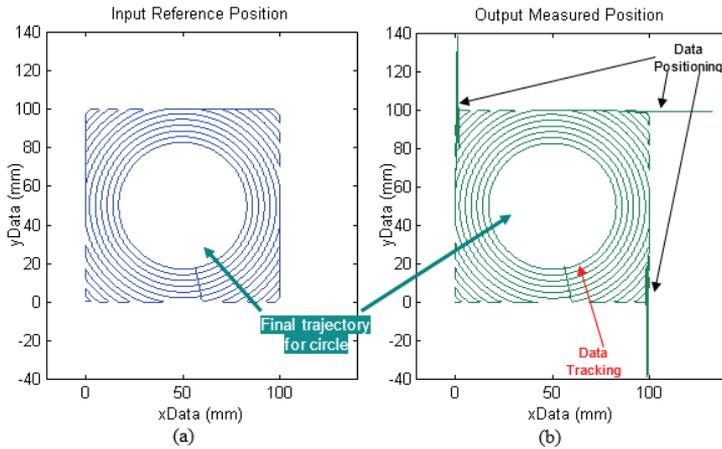
Figure 6: (a) reference tracking and (b) measured tracking data for circular contour
