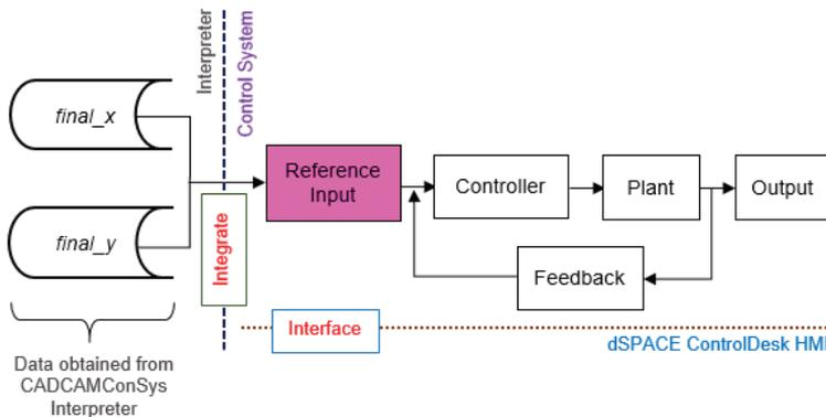
Figure 3: Integration between elements of the CAD/CAM-MATLAB/Simulink interpreter and the control system
