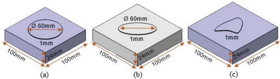
Figure 5: CATIA Drawing of a Cube with Top of (a) Circular Island, (b) Oval Island, and (c) Random-Curvy-Shaped Island
