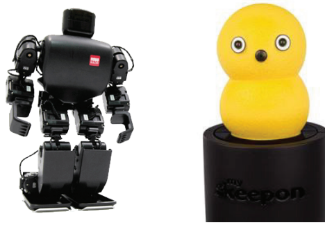
Figure 1: Robots used in this study: (a) RoboBuilder 5720T and (b) My Keepon
