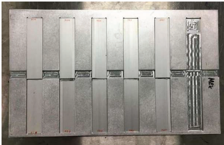
Figure 2: Sample preparation on a designed jig for lap shear test
