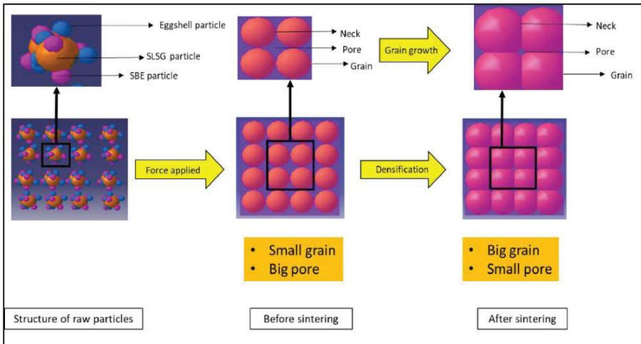
Figure 4: Illustration of model sintering process
