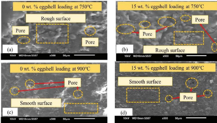
Figure 3: Fractography of fractured surface of sintered glass ceramic composite (GCC) at (a) 750 °C with 0 wt.% eggshell loading, (b) 750 °C at 15 wt.% eggshell loading, (c) 900 °C at 0 wt.% eggshell loading and (d) 900 °C at 15 wt.% eggshell loading at 500x magnification.
