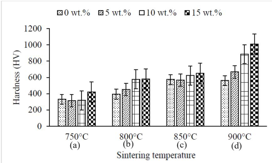
Figure 1: Hardness value of SLSW reinforced different percentage filler at different heat-treatment (sintering) temperatures (a) 750°C, (b) 800°C, (c) 850°C and (d) 900°C.
