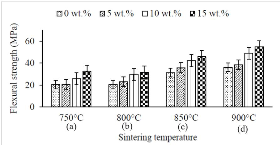
Figure 2: Flexural strength of sintered glass ceramic at different filler loading various sintering temperatures (a) 750°C, (b) 800°C, (c) 850°C and (d) 900°C.
