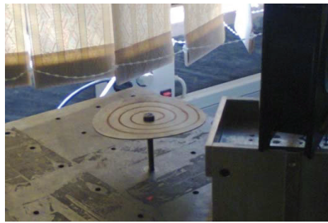
Figure 13: Spiral exposure on sheet metal
