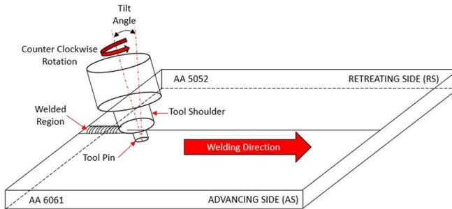
Figure 2: Illustration of FSW process and specimen setup
