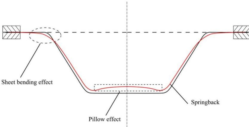
Figure 1: The common types of error found in parts produced by single-point incremental forming (SPIF) [20].
