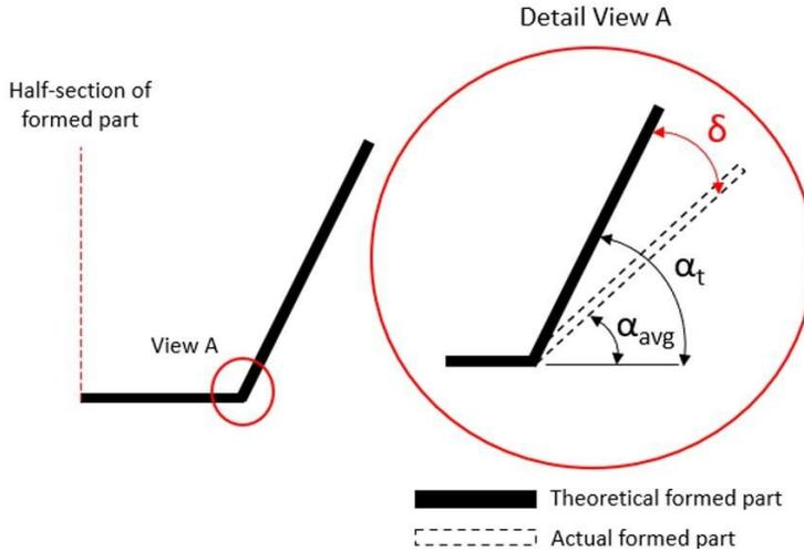
Figure 6: Schematic diagram of springback on formed part
