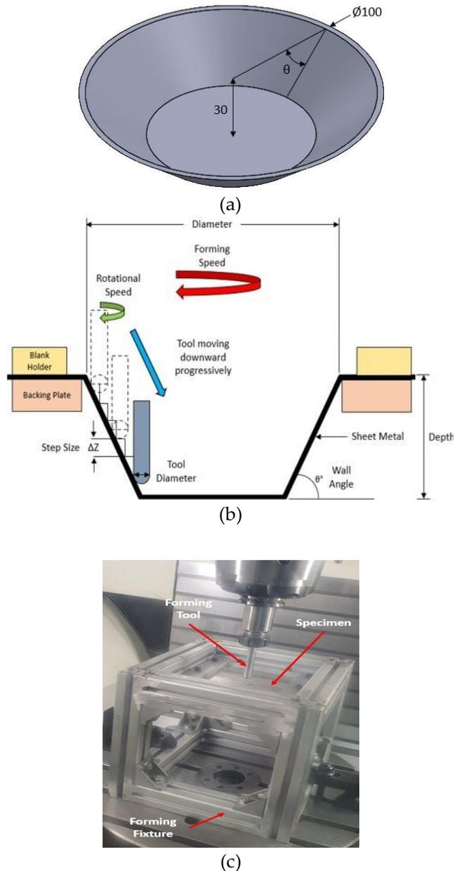
Figure 4: (a) CAD design of experiment, (b) Illustration of SPIF working principle and (c) Location of FSWed blanks on forming fixture in 5-axis CNC machine
