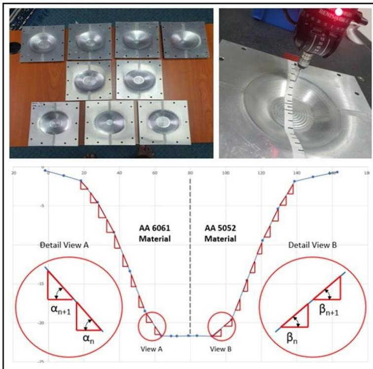
Figure 5: Measurement process on formed parts using coordinate measuring machine (CMM)
