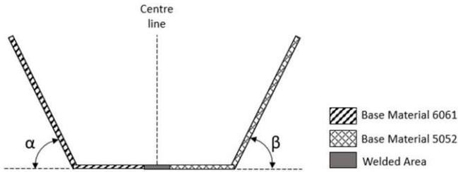
Figure 3: Illustration of measurement sections on formed dissimilar material of TWBs
