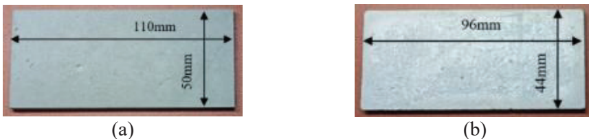
Figure 1: Conditions of SS 316L samples (a) before sintering and (b) after sintering
