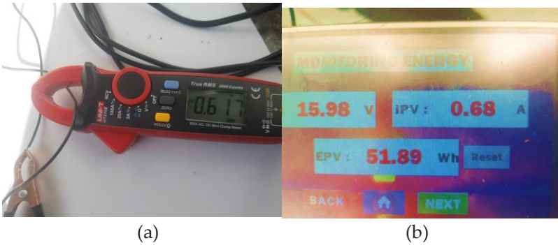
Figure 3: Calibration process (a) measurement using a standard tool, and (b) measurement of the developed system
