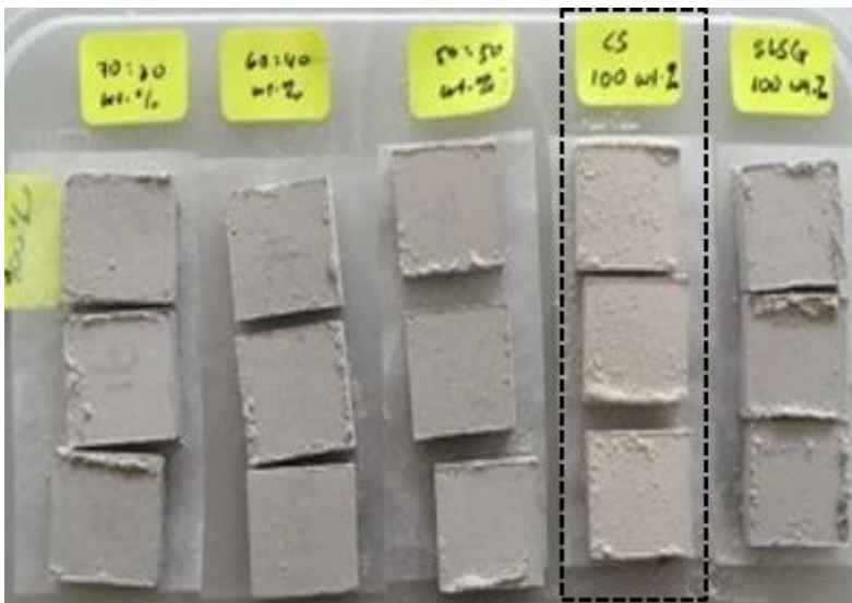
Figure 1: The green SLSG/CS composite before the sintering process
