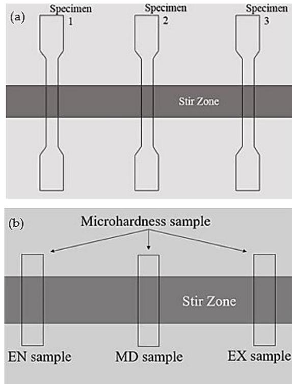
Figure 3: Arrangement of the specimens from the welded part using BFSW technique: (a) tensile specimens and (b) microhardness specimens
