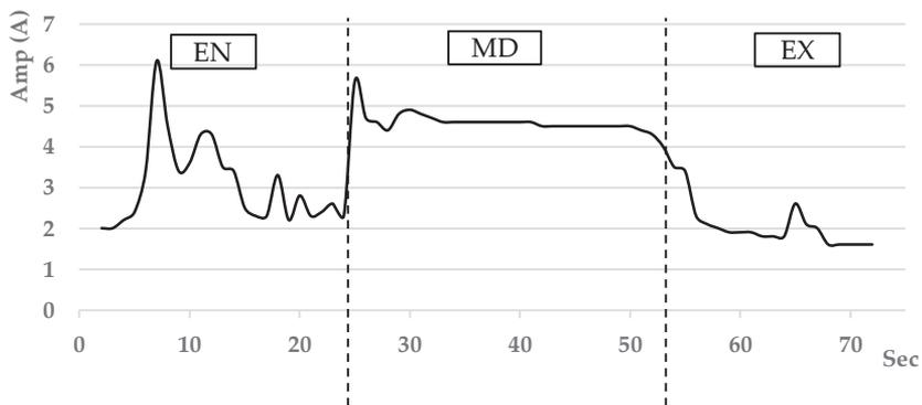
Figure 6: The recorded current along the joining process of BFSW technique at EN, MD and EX
