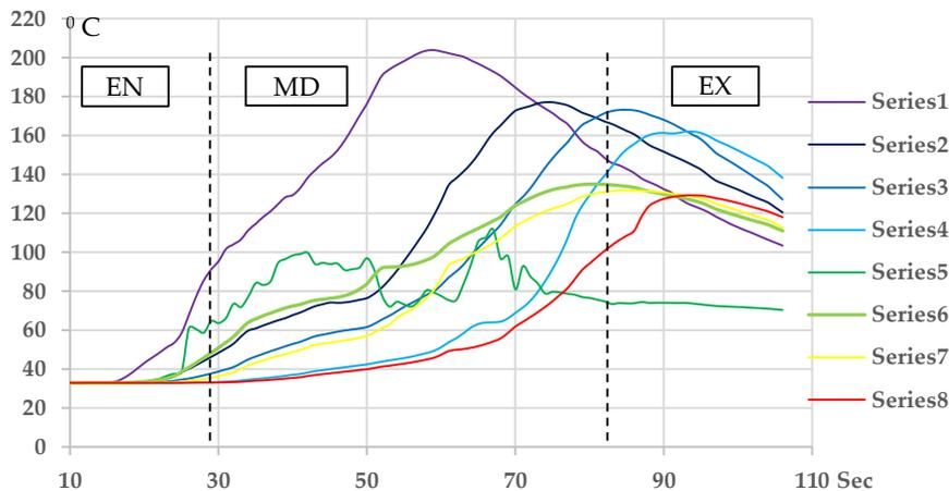
Figure 4: Temperature recorded along the weld process for EN, MD and EX
