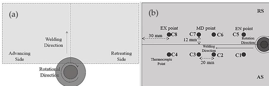
Figure 2: Process setup with (a) rotational direction,  $\omega$  is clockwise during the process and (b) location of thermocouple along the welding path
