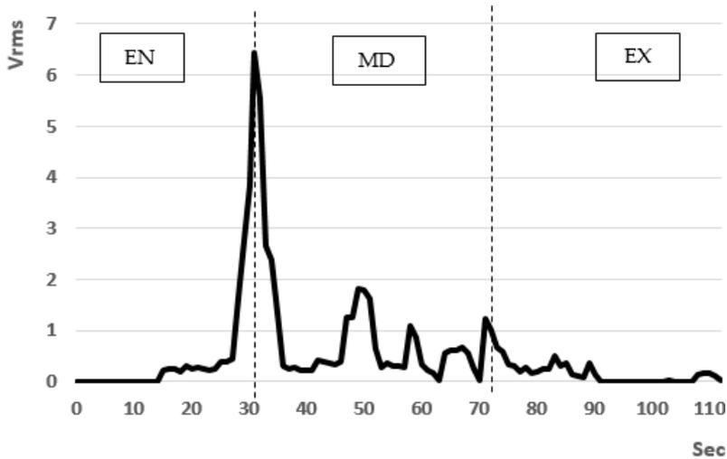
Figure 5: The vibration along the welding process at EN, MD and EX
