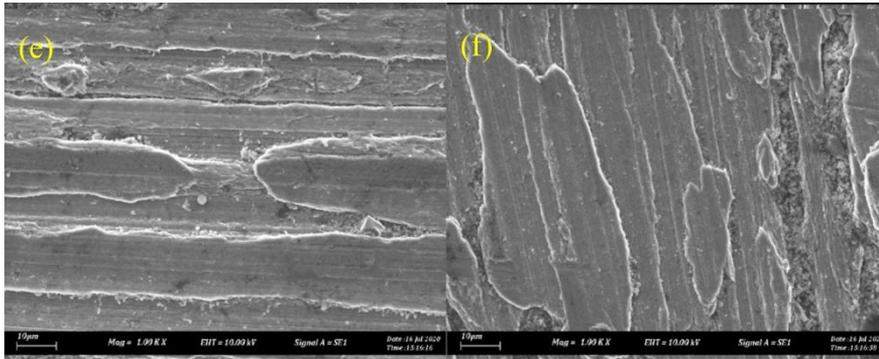
Figure 8: Microstructure of the cross-sectioned specimens: (a) SZ of the EN, (b) HAZ of the EN, (c) SZ of the MD, (d) HAZ of the MD, (e) SZ of the EX and (f) HAZ of the EX
