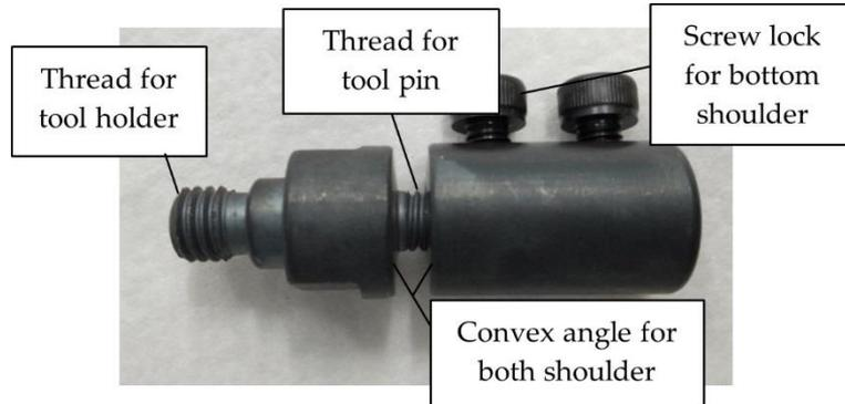
Figure 1: Bobbin tool used for experimental test
