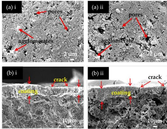
Figure 2: (a) Surface and (b) cross-sectional morphology of (i) TiO<sub>2</sub> coating, and (ii) Ag-TiO<sub>2</sub> coating, deposited on unglazed ceramic tiles
