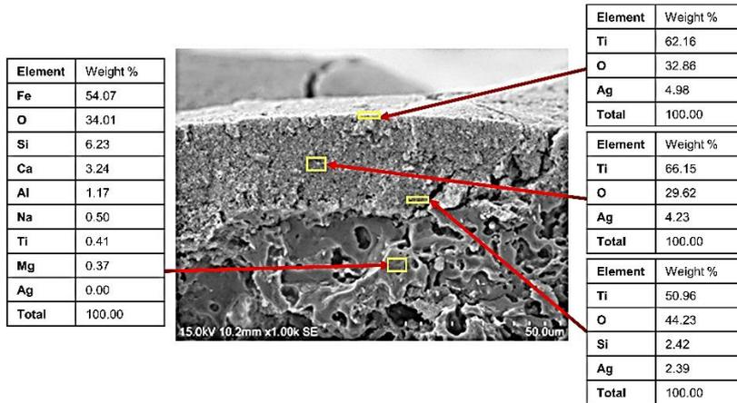
Figure 3: SEM Cross-sectional morphology and EDX spectrum of Ag-TiO<sub>2</sub> coating at 5 dipping times deposited on an unglazed ceramic tile
