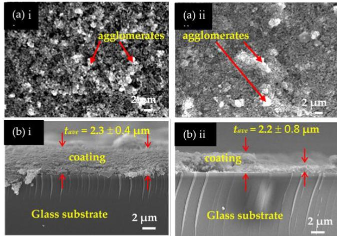
Figure 1: (a) Surface and (b) cross-sectional morphology of (i) TiO<sub>2</sub> coating, and (ii) Ag-TiO<sub>2</sub> coating, deposited on glass slides
