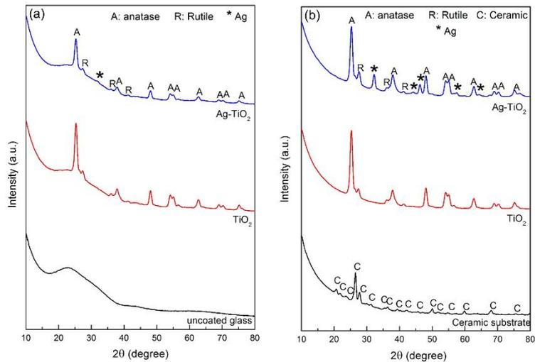
Figure 4: GAXRD diffractograms of TiO<sub>2</sub> and Ag-TiO<sub>2</sub> coatings coated at 5 dipping times deposited on (a) glass substrate and (b) unglazed ceramic tile
