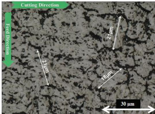
Figure 7: Image of grain size of microstructure
