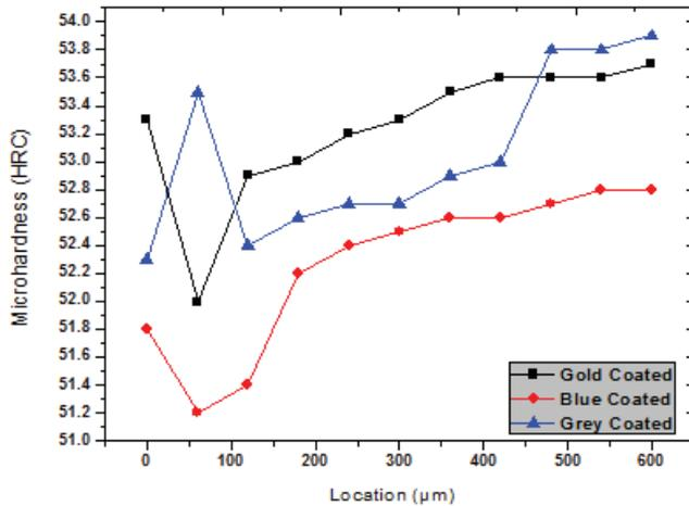
Figure 12: Graph distribution of microhardness (HRC) vs. location (µm)
