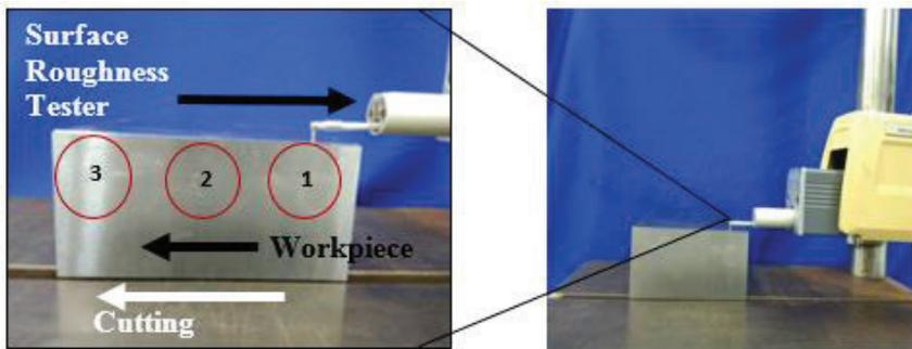
Figure 1: Image of workpiece is setup on surface roughness tester
