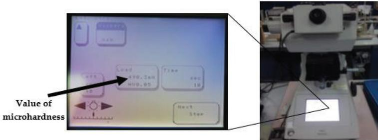
Figure 2: Value of microhardness on the screen
