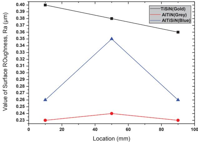
Figure 4: Graph value of surface roughness for 3 types of coated tools
