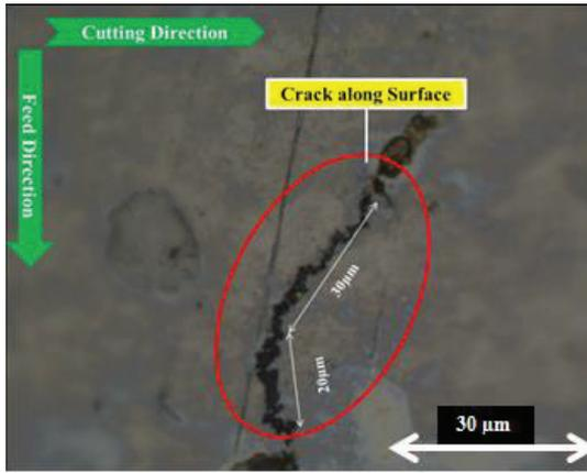
Figure 5: Image of microcrack occur along machined surface
