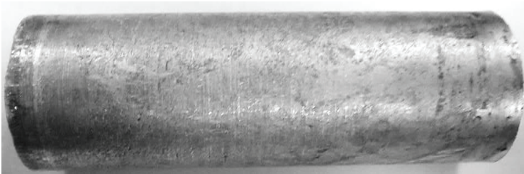
Figure 4: Billet of the sample after thixoforming
