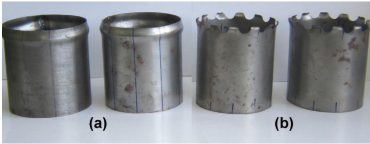
Figure 4: (a) Photograph of deformed perfect cylinders after test and (b) photograph of deformed imperfect cylinder with 12 waves after test
