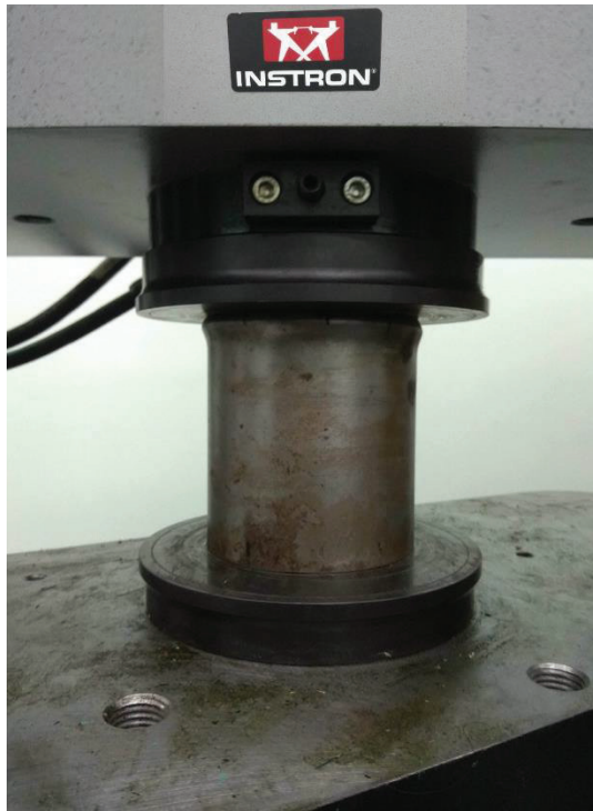
Figure 2: Experimental set-up for cylinder subjected to axial compression
