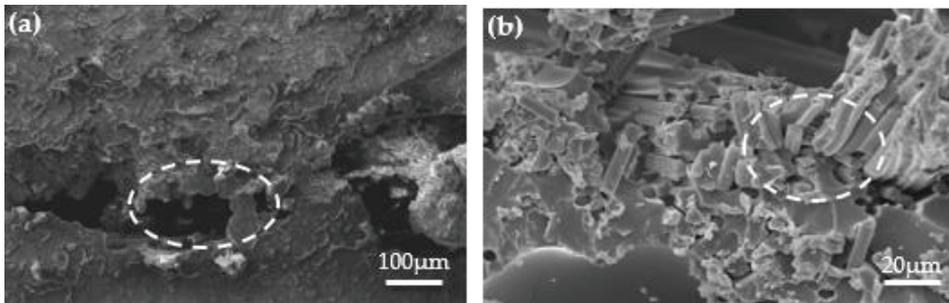
Figure 5: (a) The propagation of crack and (b) rCF breakage
