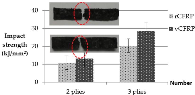
Figure 4: Izod impact strength of rCFRP and vCFRP for different ply with features of fracture after tested
