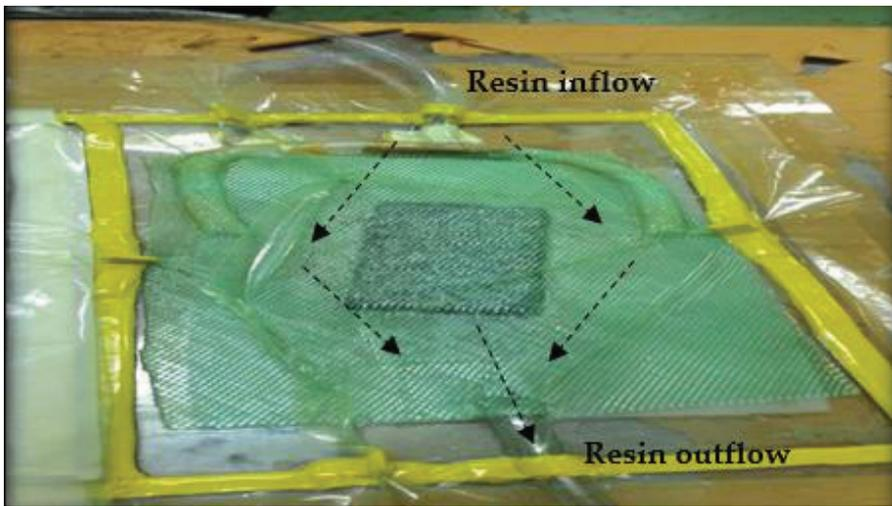
Figure 3: The flowability of resin from inlet to outlet of vacuum infusion process
