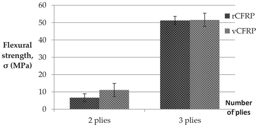
Figure 2: Flexural strength for sample rCFRP and vCFRP
