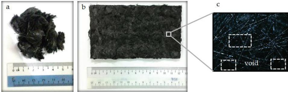
Figure 1: The rCF nonwoven mat after wet-laid process of (a) fluffy rCF, (b) nonwoven mat and (c) micrograph of rCF distribution via optical microscopy
