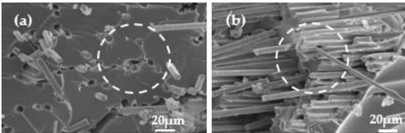
Figure 7: (a) The failure mode of fibre pull-out and (b) rCF breakage
