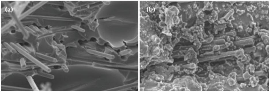
Figure 6: (a) The fibres pull-out and breakage while (b) rCF appeared when not fully coated by epoxy
