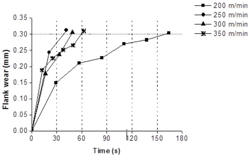
Figure 4: Effect of cutting speed when machining alumina-zirconia cutting tool with AISI 1045 at the feed rate of 0.175 mm/rev
