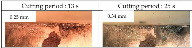
Figure 5: Wear development for alumina based cutting tool at the cutting speed of 350 m/min and 0.175 mm/rev feed rate
