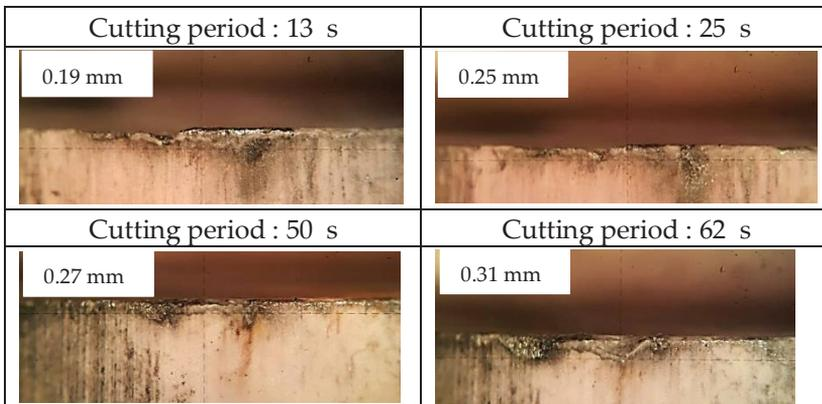
Figure 6: Wear development for alumina-zirconia based cutting tool at the cutting speed of 350 m/min and 0.175 mm/rev feed rate
