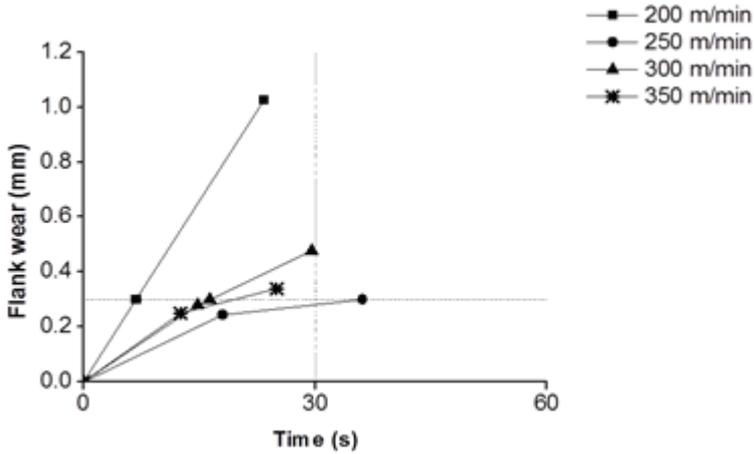
Figure 3: Effect of cutting speed when machining alumina cutting tool with AISI 1045 at the feed rate of 0.175 mm/rev
