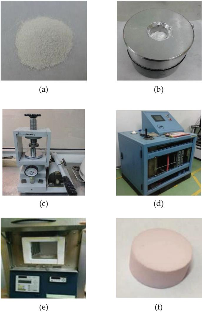
Figure 1: Procedure to fabricate alumina-zirconia cutting tool started with (a) blending alumina and zirconia powders, (b) inserting the powders into the mould, (c) pressing the mould by hydraulic, (d) pressing the mould by using cold isostatic press, (e) sintering the compacted powders to obtain ceramic cutting tool and (f) solid sintered of ceramic cutting tool
