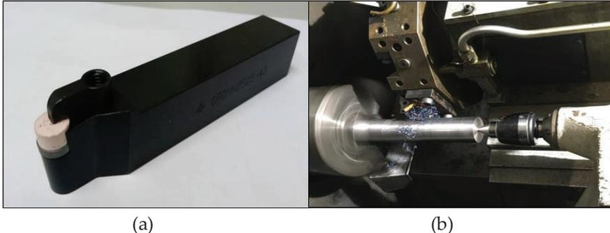
Figure 2: (a) Cutting tool with the design of RNGN120600 clamped in CRDN252543 tool holder and (b) machining setup with AISI 1045 workpiece
