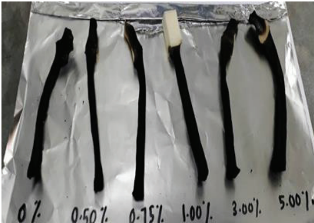
Figure 4: Burnt samples after UL-94 flame retardant test of PU/bentonite composite foams
