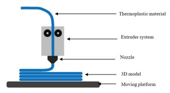
Figure 1: Schematic diagram of FDM technique
