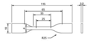
Figure 2: Dimension of testing specimen according to ASTM D638
