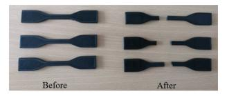
Figure 3: Specimens before and after the tensile test
