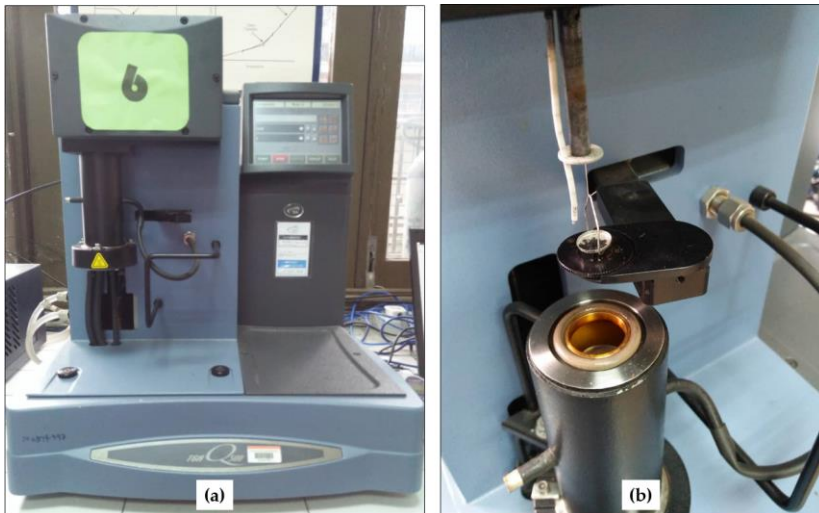
Figure 4: TGA analysis: (a) thermal analyser and (b) sample loading
