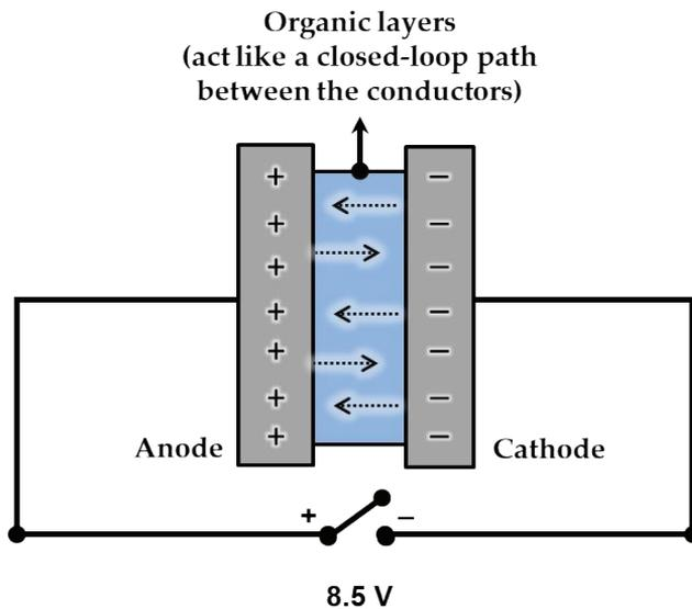
Figure 5: Organic layer acted like a closed-loop path to allow the charge balance process within the OLED device to occur (as indicated by the dashed arrows)
