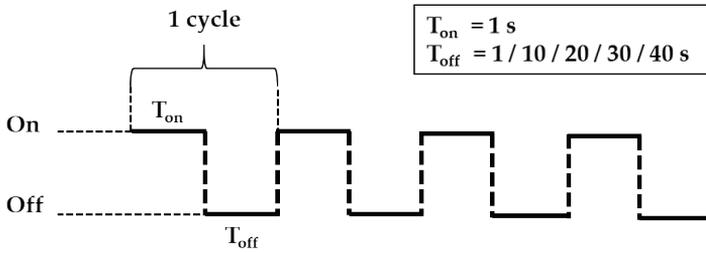
Figure 2: Cyclic diagram of the on/off cycles approach at fixed  $T_{on}$  and different  $T_{off}$
