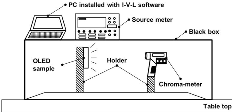
Figure 3: Schematic diagram of the in-house black-box setup
