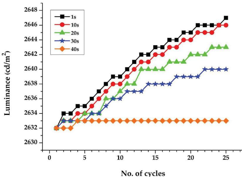
Figure 4: Performance of luminance outputs over cycles at different  $T_{\text{off}}$
