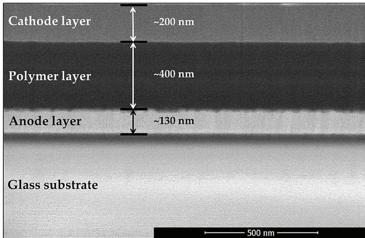
Figure 1: Configuration of the OLED sample
