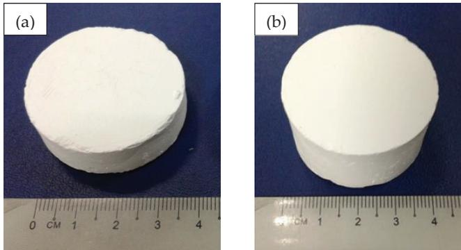
Figure 3: Zirconia blocks produced through slip casting and CIP: (a) 20 nmZ with thickness 5 mm and (b) 60 nmZ with thickness 20 mm
