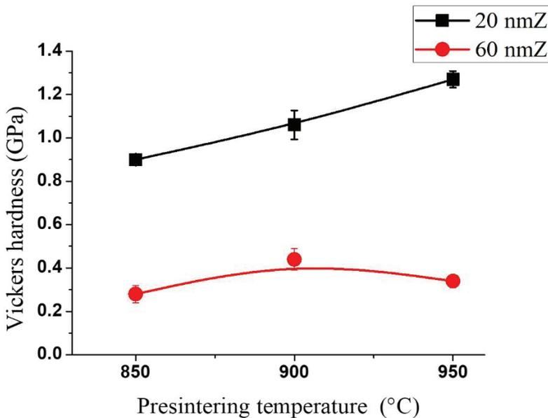
Figure 6: Vickers hardness of zirconia block at different pre-sintering temperatures
