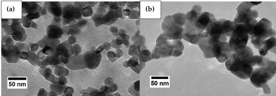
Figure 1: TEM images of (a) 20 nmZ and (b) 60 nmZ powders
