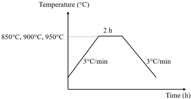
Figure 2: Sintering profile of the block samples
