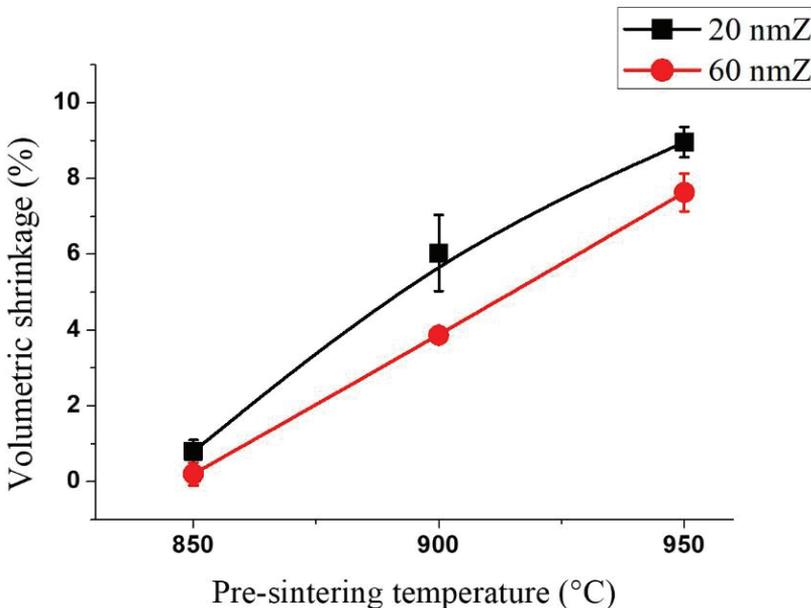
Figure 4: Volumetric shrinkage of zirconia block at different pre-sintering temperatures
