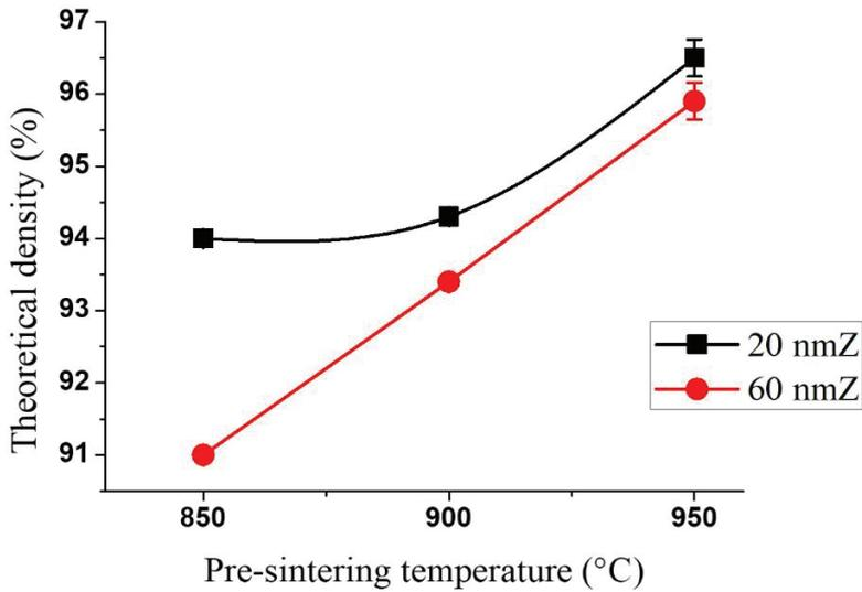
Figure 5: Theoretical density of zirconia block at different pre-sintering temperatures
