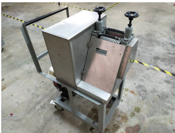
Figure 2: PALF breaker machine
