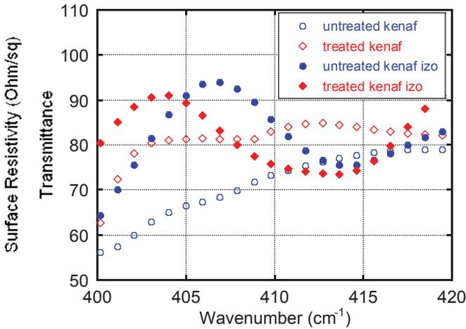
Figure 5: A close-up FTIR spectra showing the peak associated to Zn-O at 410-415  $\text{cm}^{-1}$
