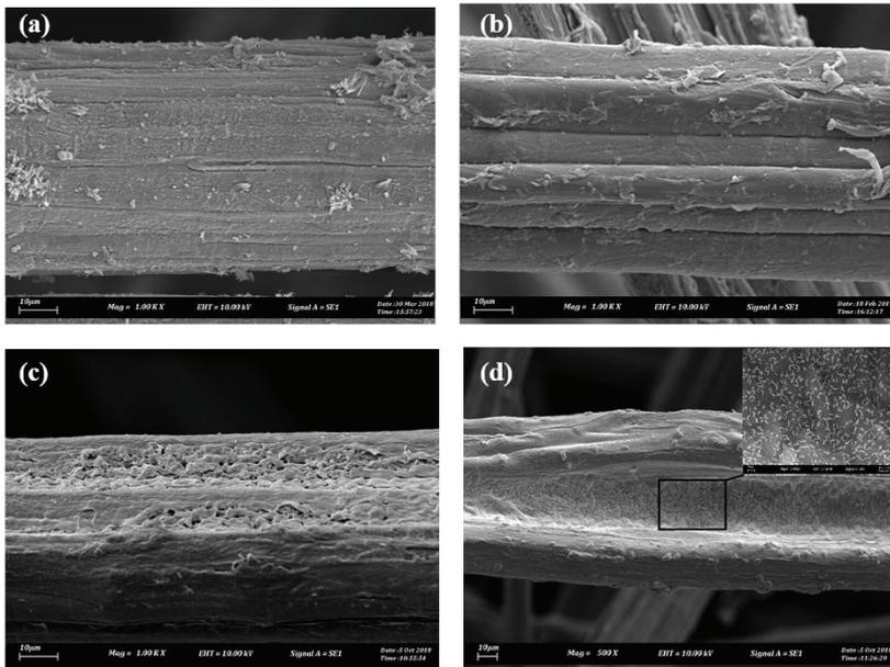
Figure 1: SEM images of (a) neat kenaf, (b) NaOH treated kenaf, (c) IZO coated untreated kenaf and (d) IZO coated NaOH treated kenaf
