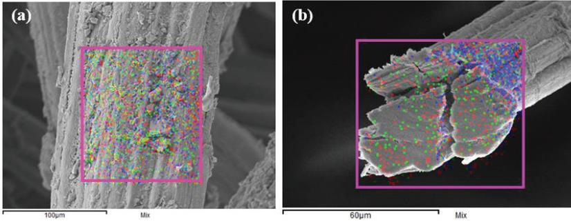
Figure 2: SEM-EDX analysis of IZO coated kenaf fiber on (a) surface and (b) cross section of fiber
