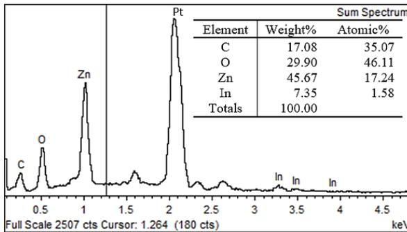
Figure 3: EDX spectrum of IZO coated kenaf fiber with percentage of each element for 5 at% of indium doping
