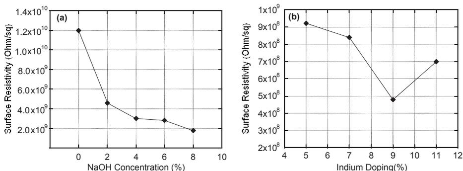
Figure 6: Effects of (a) NaOH concentration and (b) Indium doping on surface resistivity of IZO coated kenaf
