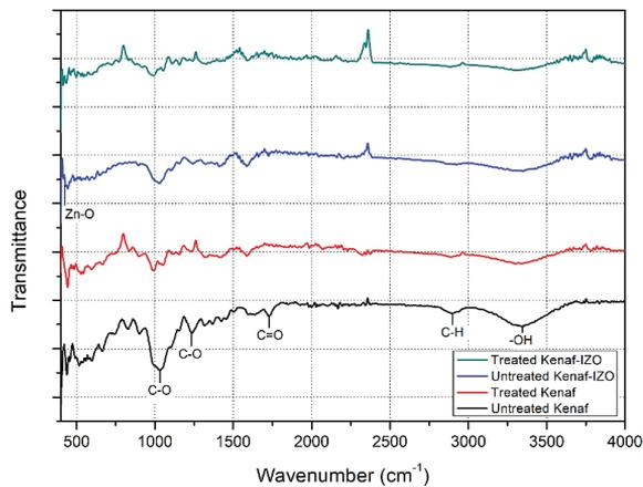
Figure 4: FTIR spectroscopy patterns of untreated kenaf, treated kenaf, untreated kenaf-IZO and treated kenaf-IZO samples
