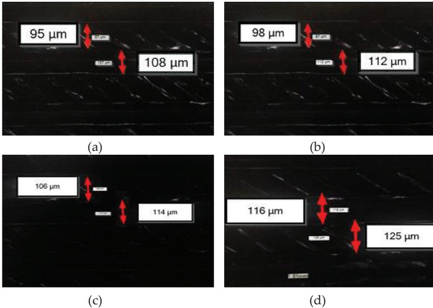
Figure 5: Actual lines width results produced by Myvista Cube 200 printer:
