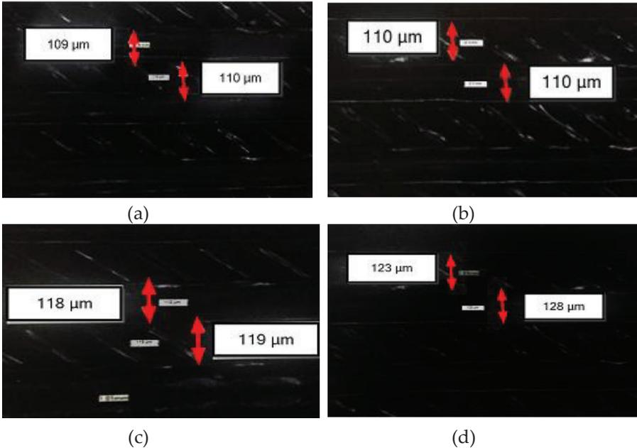
Figure 4: Actual lines width results produced by Raise Pro N2 Plus printer:
