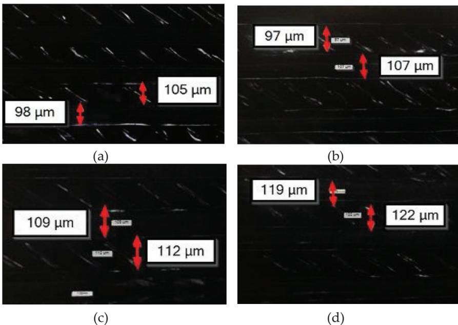
Figure 3: Actual lines width results produced by Cubicon Single 3DP-110F printer: (a) square spiral shape with a 100 μm width and gap, (b) straight lines pattern of 100 μm width and gap, (c) straight lines pattern of 110 μm width and gap and (d) straight lines pattern of 120 μm width and gap
