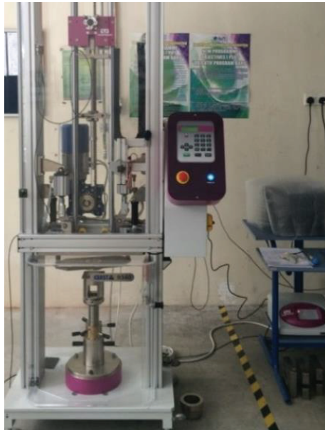
Figure 1: An experimental set-up for drop weight impact test using an INSTRON CEAST 9340 machine
