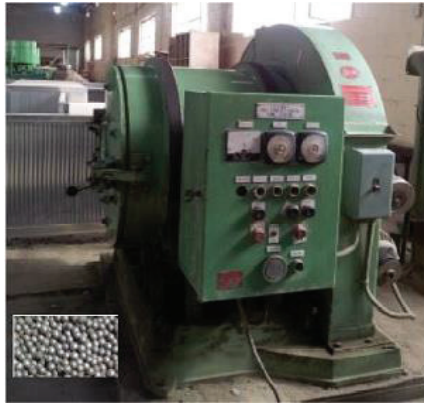
Figure 3: Shot peening device with shot balls
