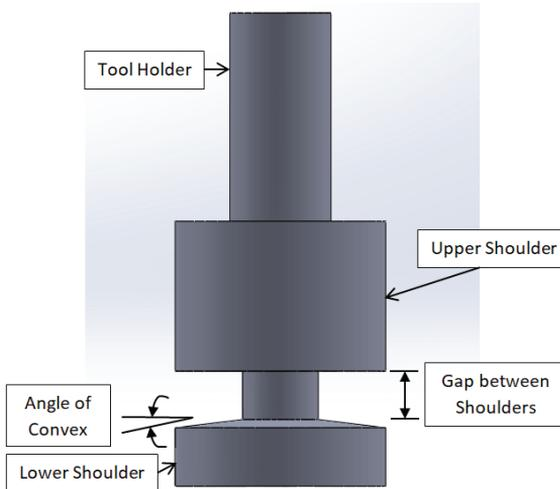
Figure 1: Drawing of bobbin tool
