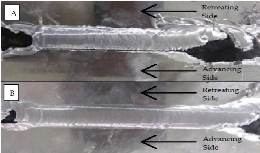
Figure 3: Welding quality for 6 mm thickness plate: (A) Tool 1 with 7° tapered and (B) Tool 2 with 5° tapered
