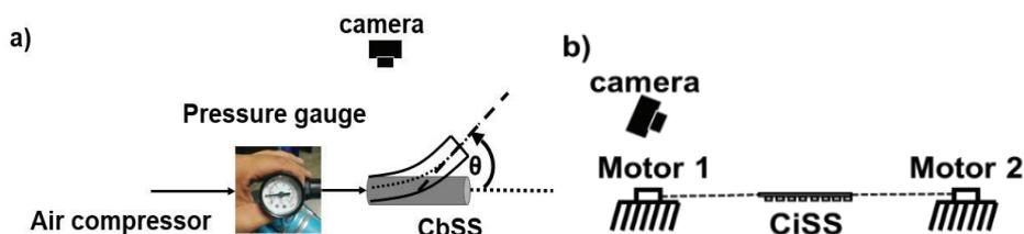
Figure 5: Experimental setups to test soft robotic structures: (a) CbSS deformation and (b) CiSS locomotion: two servo motors
