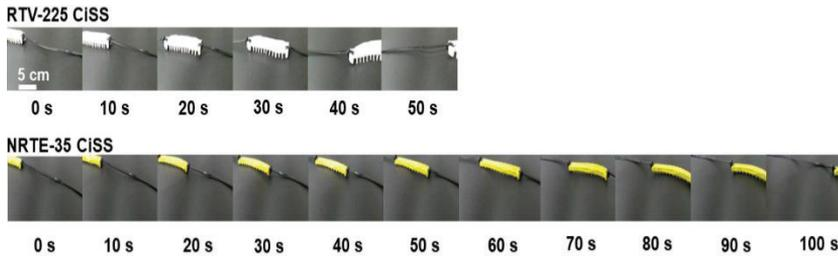
Figure 7: The experimental locomotion of RTV-225 (top) and NRTE-F35 (bottom) CiSS structures
