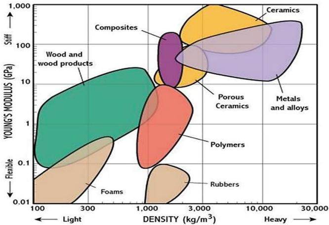
Figure 1: Material selection chart illustrating choice of materials based on density and Young's modulus [21]
