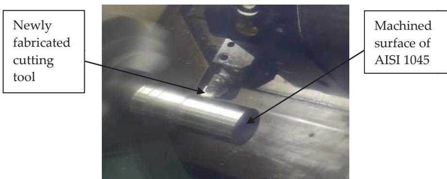
Figure 4: Alumina cutting tool on tool holder when machining AISI 1045
