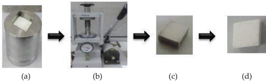
Figure 3: The compaction method procedures: (a) Powder pours into the mould, (b) The mould is pressed by hydraulic hand press, (c) The body is ejected out from the mould and (d) Ceramic cutting tool after sintering the white body colour
