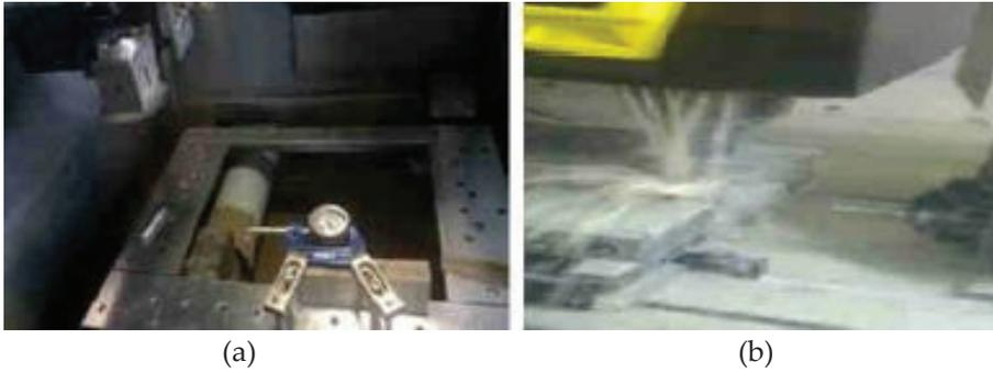
Figure 1: Mould machining process: (a) Wire cut machine and (b) CNC milling
