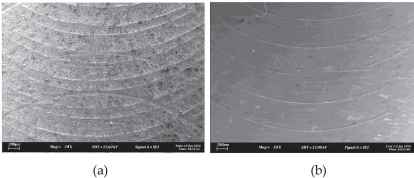
Figure 7: Cutter marks formation for (a) conventional milling and (b) RUAM
