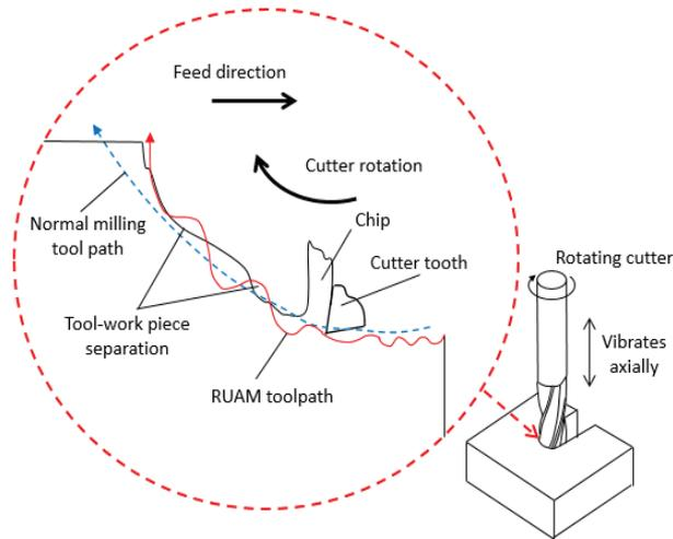
Figure 1: Mechanics of RUAM material removal process
