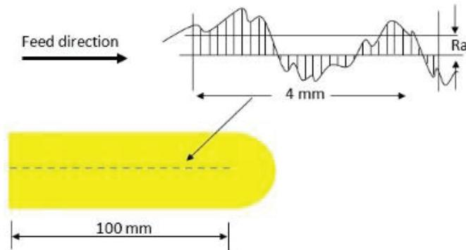
Figure 3: Surface roughness measuring location
