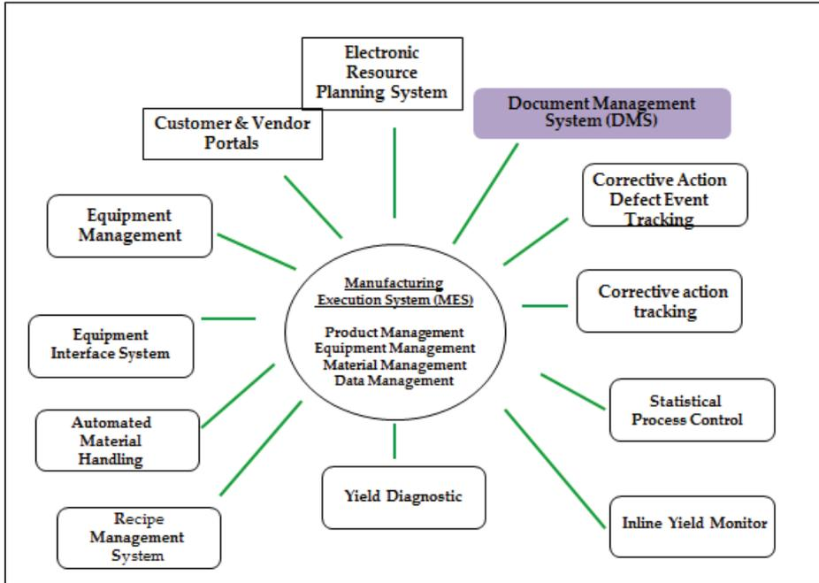
Figure 1: Interlinked manufacturing execution system
