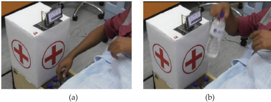
Figure 10: (a) Water bottles placed in the front rack of the robot and (b) The bottles are easily accessible to the patients from the bed
