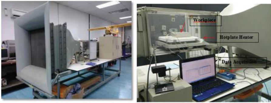
Figure 2: The setup of experiment in wind tunnel
