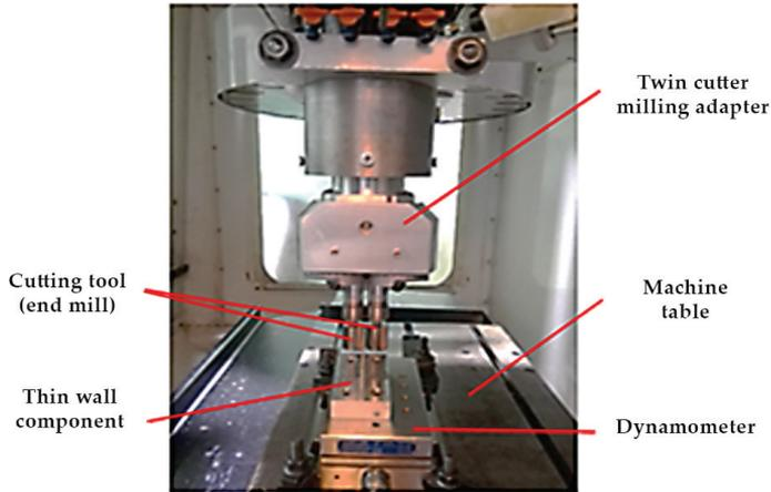
Figure 7: Experimental setup
