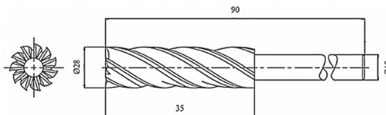
Figure 8: End mill specification for twin cutter adapter
