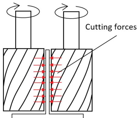
Figure 2: Act of cutting force in twin cutter machining technique
