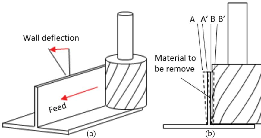
Figure 1: Un-cut materials in machining thin-wall feature
