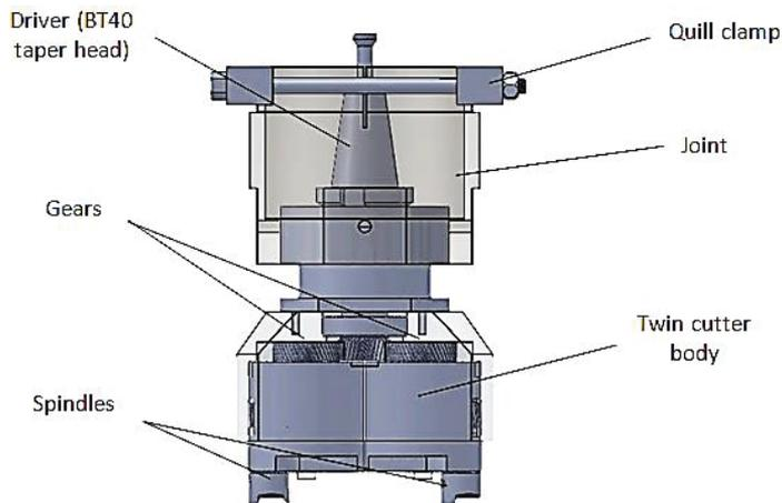
Figure 3: Principle of twin cutter machining technique
