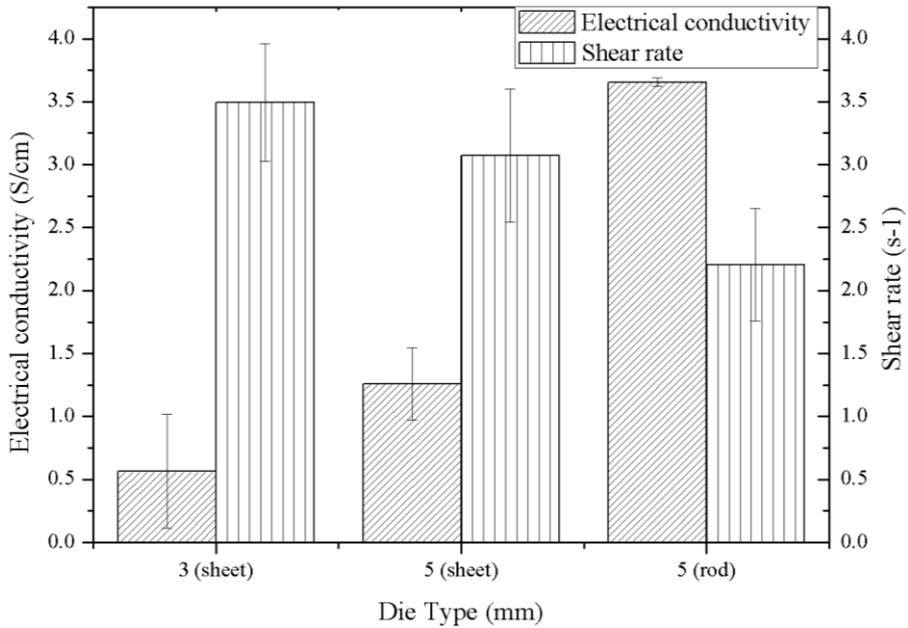
Figure 2: Electrical conductivity and shear rate of MCF/PP composites
