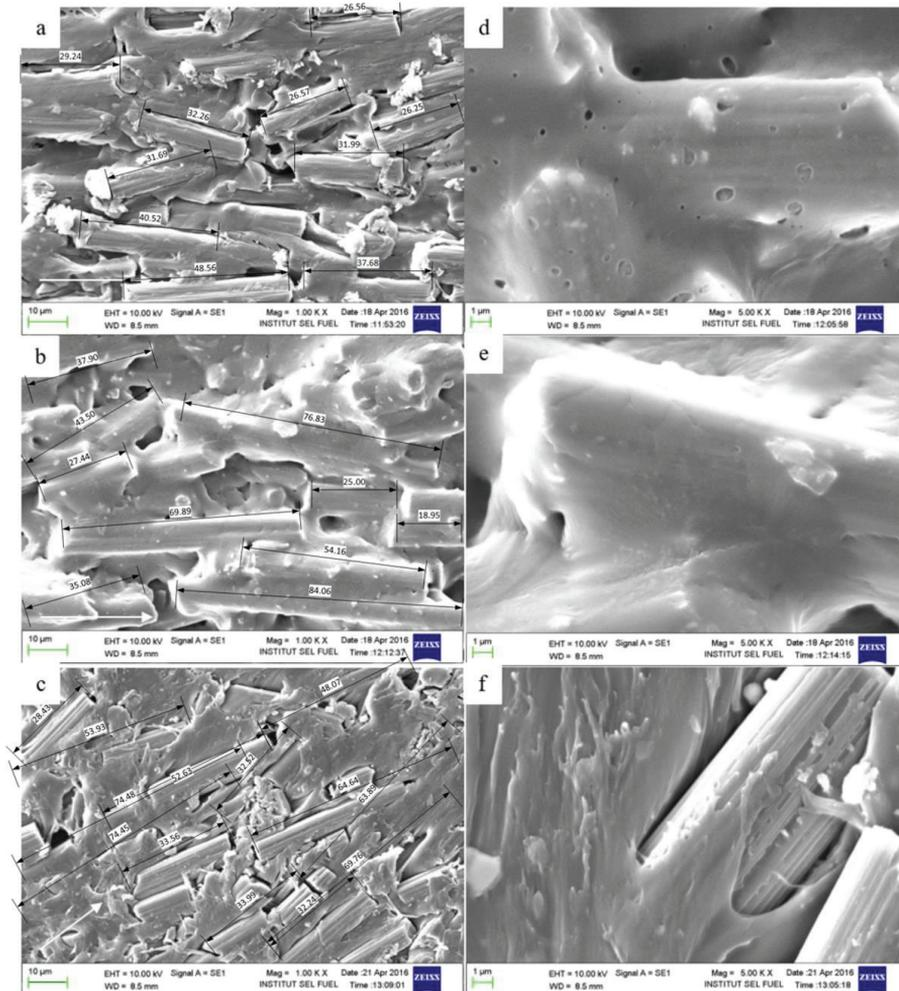
Figure 3: 1.0K SEM image magnification of fibre length of (a) 3mm thick sheet die, (b) 5mm thick sheet die and (c) 5mm wide of rod die while 5.0K SEM image magnification of (d) 3mm thick sheet die, (e) 5mm thick sheet die and (f) 5mm wide rod die
