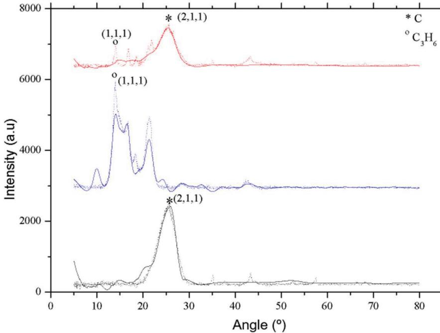
Figure 1: XRD analysis of extruded raw MCF, raw PP and MCF/PP composite
