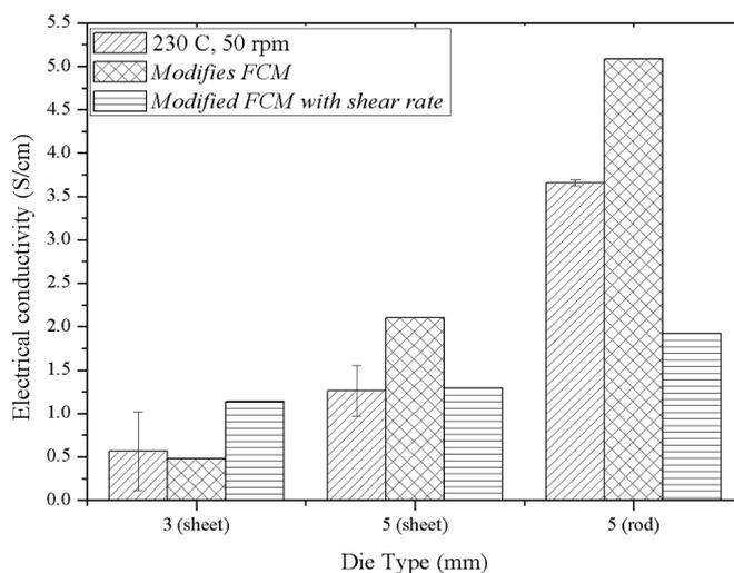
Figure 4: Electrical conductivity of extruded MCF/PP composites and electrical conductivity predicted using modified FCM model
