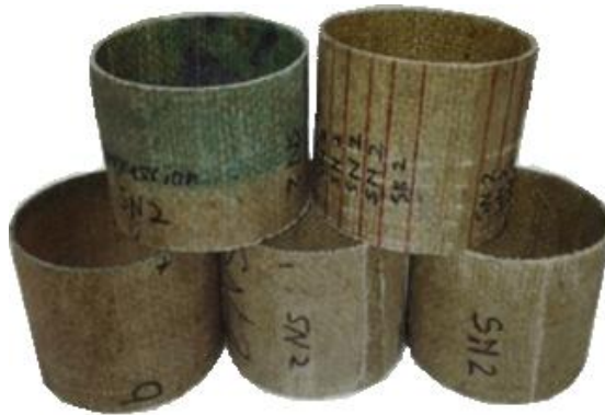
Figure 4: Jute pipe structure
