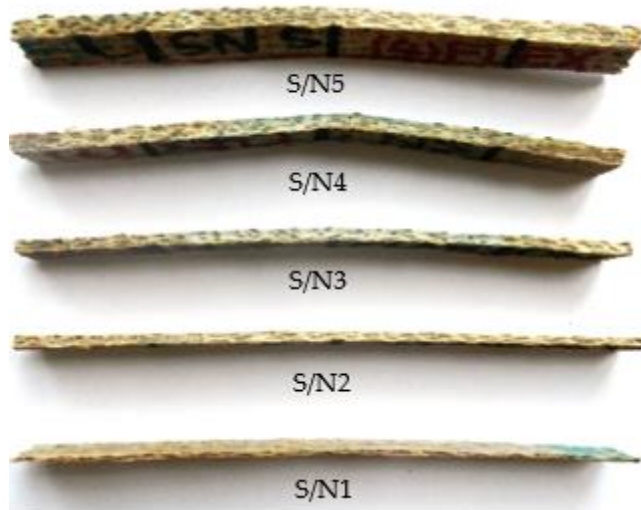
Figure 13: Five samples after tested under flexural load
