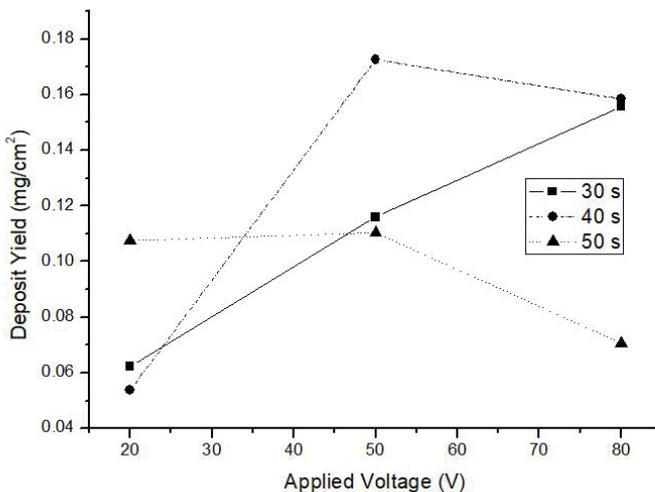
Figure 3: Deposit yield of CNT coatings deposited at different pulse separation times as function of applied voltage
