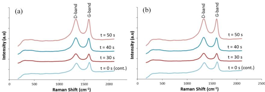
Figure 5: Raman spectra of: (a) AC and (b) CNT deposit formed by pulsed EPD at different pulse separation times and applied voltage of 80 V ( $t = 0$  s refers to deposit formed by EPD at a continuous deposition time of 10 min)
