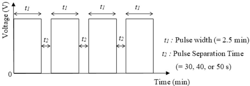
Figure 1: Pulsed EPD process's pulsed voltage–time profile
