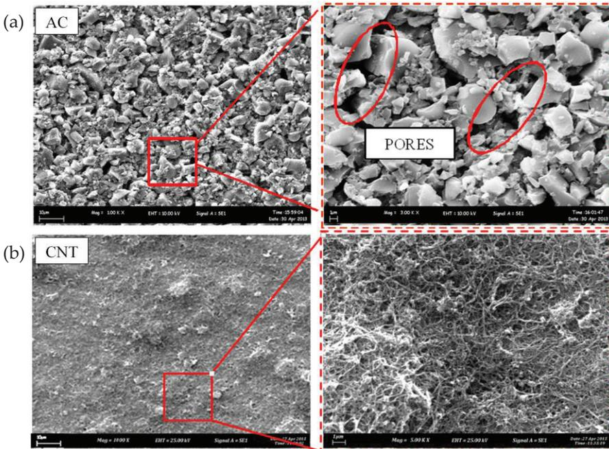
Figure 4: SEM surface images of (a) AC and (b) CNT coatings deposited by EPD at constant 80 V for a continuous 10 min
