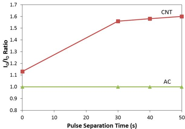
Figure 6: G-band /D-band peak intensity ratio of CNT and AC coatings deposited at different pulse separation time (applied voltage = 80 V)
