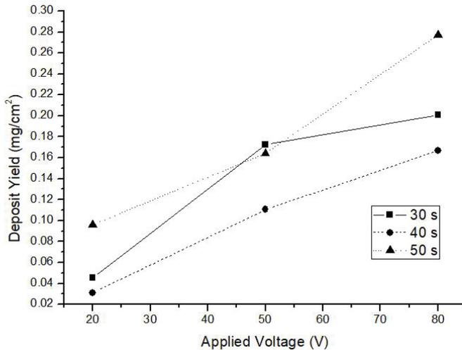
Figure 2: Deposit yield of AC coatings deposited at different pulse separation times as function of applied voltage
