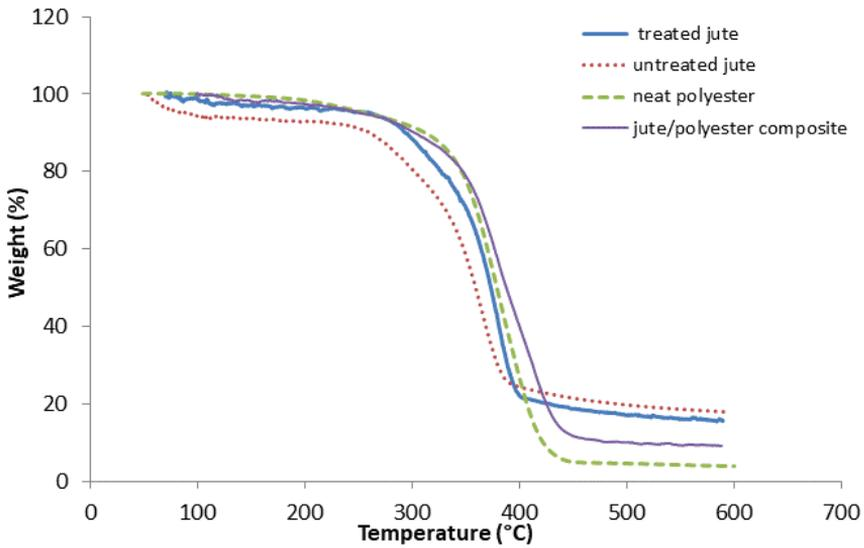
Figure 1: TGA analysis of neat resin, jute fibres and woven jute/polyester composite
