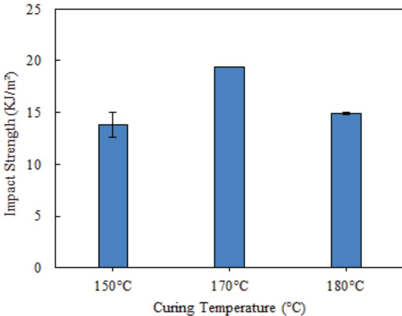
Figure 3: Effect of curing temperature on Charpy impact properties of jute/polyester composite
