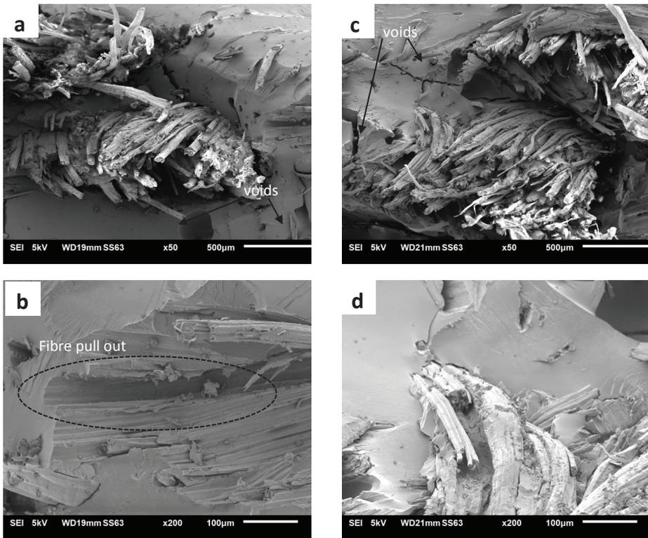
Figure-4. SEM micrographs of Charpy impact fracture of 40 vol.% jute/unsaturated polyester composites cured at (a)-(b) 150°C and (c)-(d) 170°C
