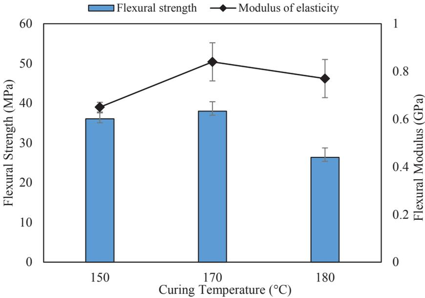
Figure 2: Effect of curing temperature on flexural properties of jute/polyester composite
