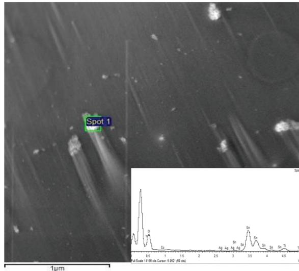
Figure 5: HRTEM micrographs of an ultra-fine solder joint (lead-free Sn-3.0Ag-0.5Cu-TiO<sub>2</sub> composite solder) and EDS pattern results that indicated in the spot region (Spot 1)
