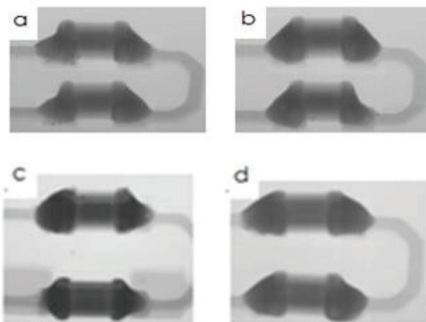
Figure 3: Laminography X-ray images (400 $\times$ ) of ultra-fine joints: (a) lead-free Sn-3.0Ag-0.5Cu- 0.01TiO<sub>2</sub>, (b) lead-free Sn-3.0Ag-0.5Cu-0.05TiO<sub>2</sub>, (c) lead-free Sn-3.0Ag-0.5Cu- 0.15TiO<sub>2</sub> and (d) plain lead-free Sn-3.0Ag-0.5Cu only
