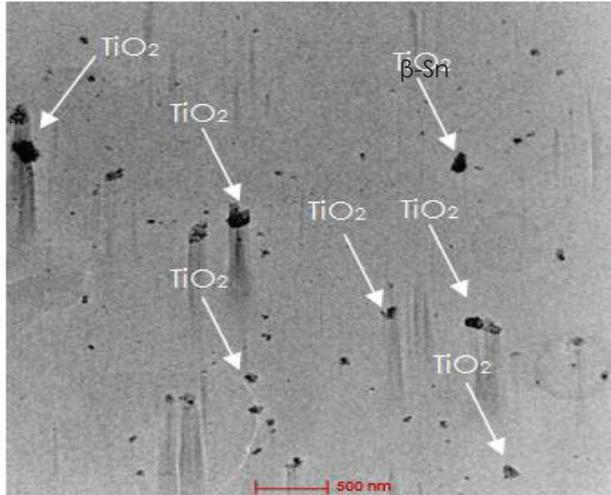
Figure 4: HRTEM micrographs of an ultra-fine solder joint
