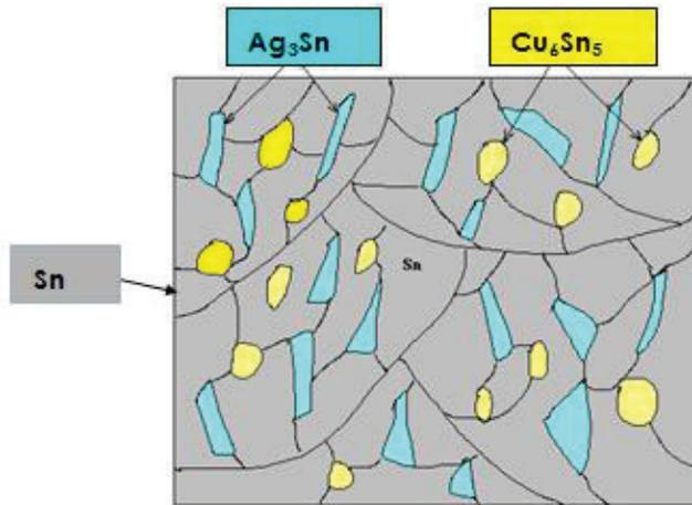
Figure 7: Schematic diagram of typical eutectic Sn-Ag-Cu structure
