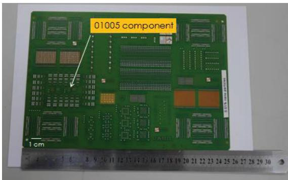
Figure 2: Reflowed PCB with ultra-fine package component
