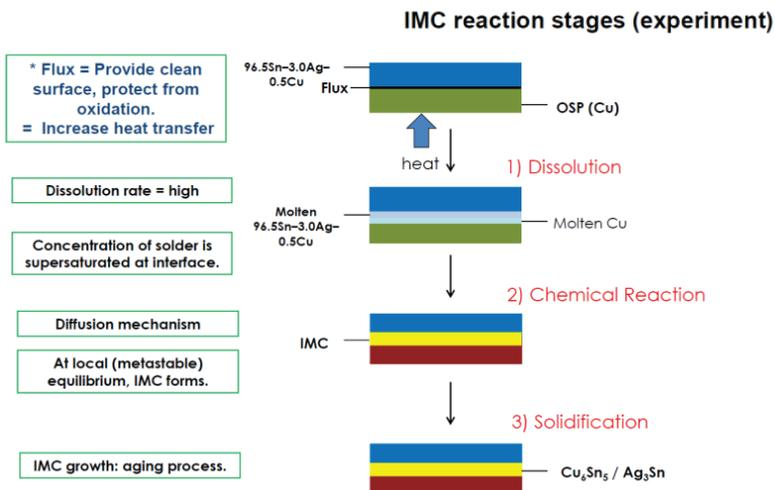
Figure 6: Schematic diagram of the IMC reaction stages under reflow process
