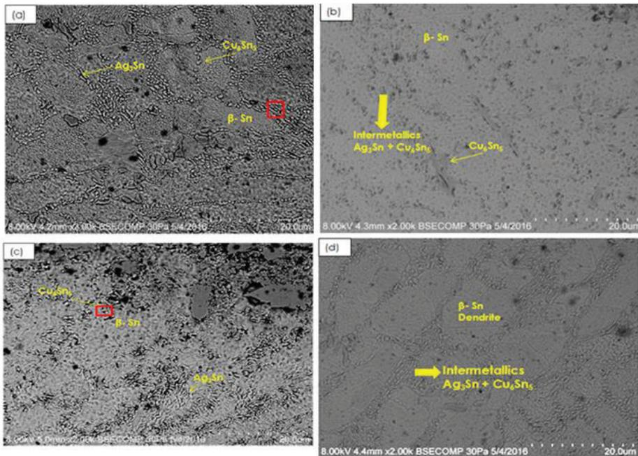
Figure 8: Scanning electron microscope backscattered electron of the cross-sectioned matrix for (a) lead-free Sn-3.0Ag-0.5Cu-0.01TiO<sub>2</sub>, (b) lead-free Sn-3.0Ag-0.5Cu-0.05TiO<sub>2</sub>, (c) lead-free Sn-3.0Ag-0.5Cu-0.15TiO<sub>2</sub> and (d) plain lead-free Sn-3.0Ag-0.5Cu
