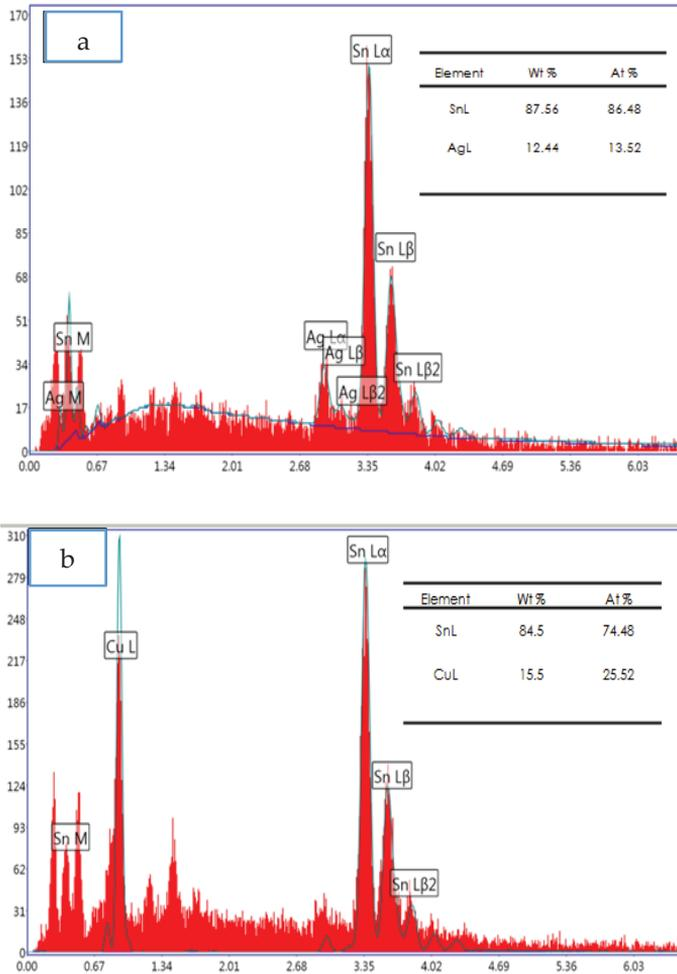
Figure 9: (a) EDS pattern for Ag<sub>3</sub>Sn and (b) EDS pattern for Cu<sub>6</sub>Sn<sub>5</sub> in the scan area
