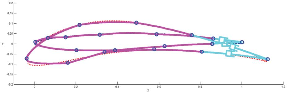
Figure 6: The wing with 10 segments approximating two profiles
