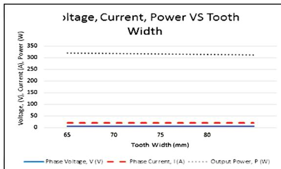
Figure 4: Voltage, Current and Power vs Tooth width of stator
