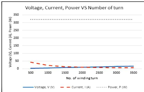
Figure 2: Voltage, Current and Power vs No. of turns
