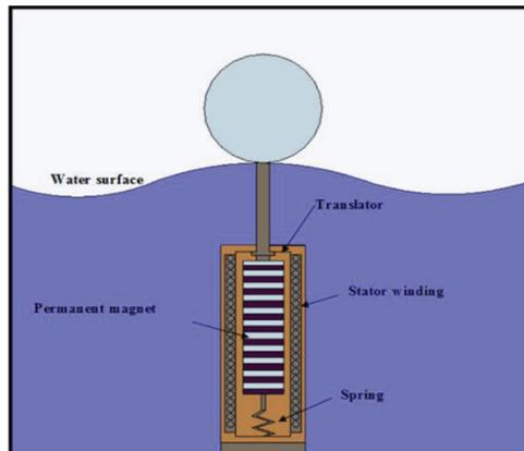
Figure 1: Schematic diagram of wave energy converter
