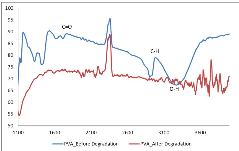
Figure 2 : FTIR spectra from PVA particles before and after degradation process
