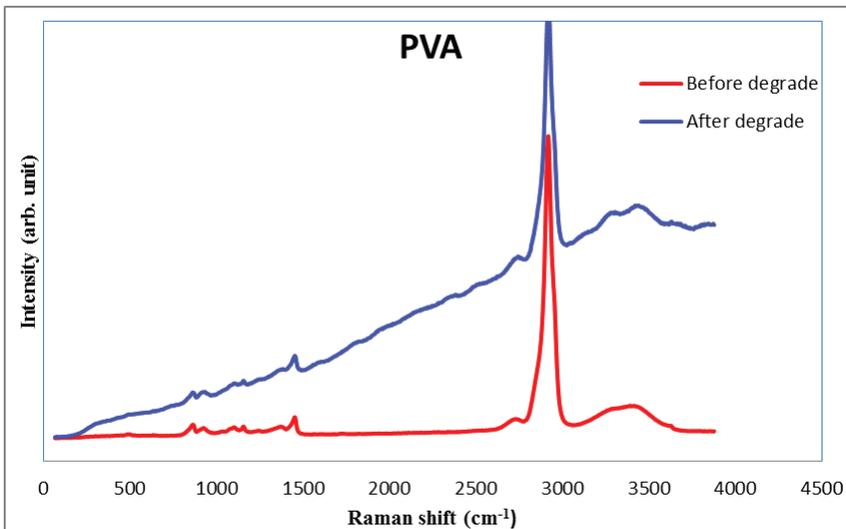
Figure 3 : Raman spectrum of PVA before and after biodegradation
